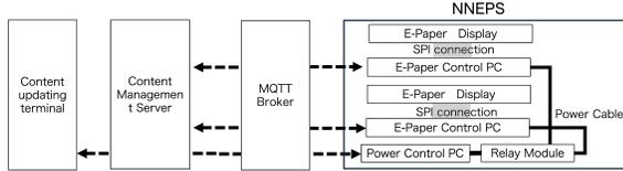
Figure 3. Configuration chart of the NNEPS System
